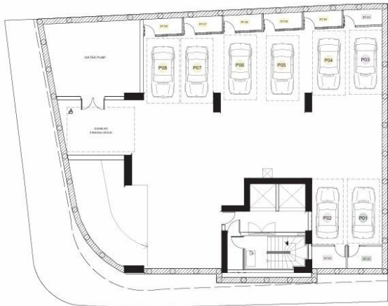
-2 BASEMENT PLAN SCALE 1:100
