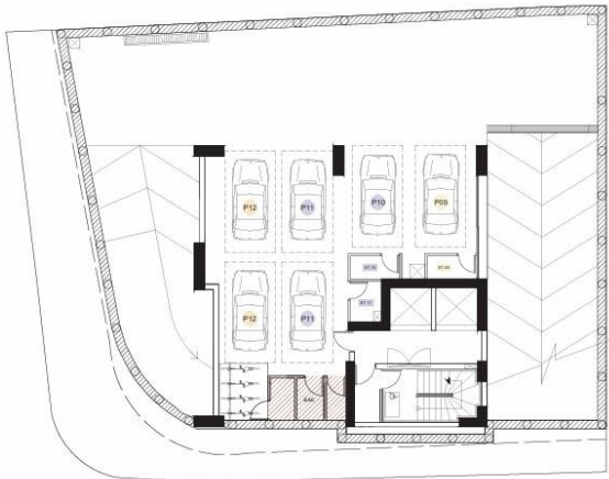
-1 BASEMENT PLAN SCALE 1:100
